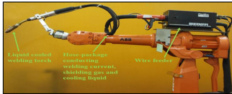
Figure 4. Robotic Arm Welding ABB IRB 2400/16 with GMAW Kemmpil Pro-Evolution ProMIG 540 MX
