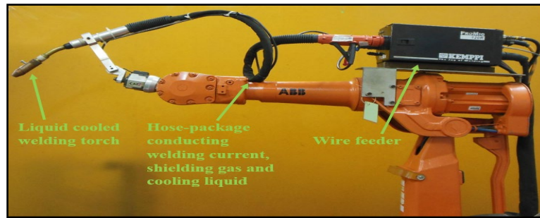
Figure 4. Robotic Arm Welding ABB IRB 2400/16 with GMAW Kemppi Pro-Evolution ProMIG 540 MX
