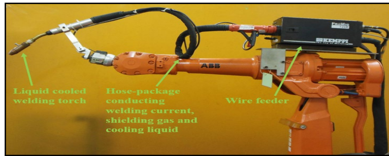
Figure 4. Robotic Arm Welding ABB IRB 2400/16 with GMAW Kemppil Pro-Evolution ProMIG 540 MX
