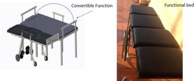
Figure 6. The new design wheelchair (Functionality)
