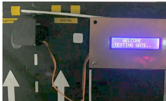
Figure 12: LCD Screen shown Testing Gate Command.
